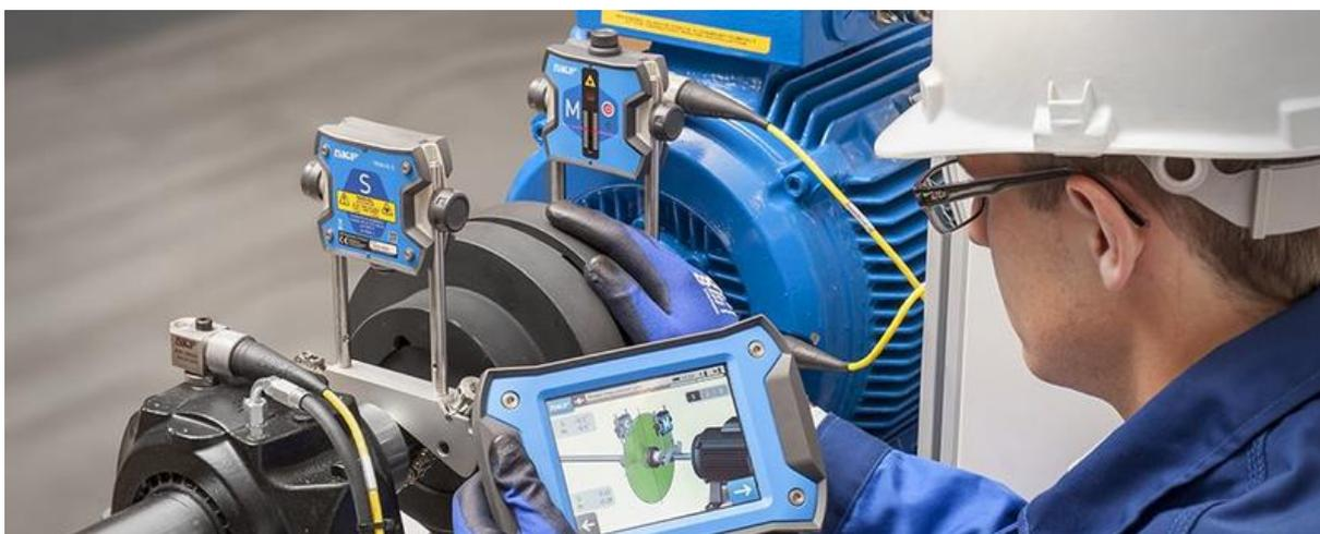
**Figura 19** – Alinhador a laser. ([www.skf.com](http://www.skf.com))
